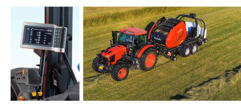
The proven, AEF-certified 7" K-Monitor is available as an option for the M6002. ISOBUS capability and an optional automatic steering system makes the tractor ready for precision farming. Enabling precise use of resources and efficient headland management.
